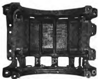
Fig. 4659. Interior of Gearless Motor Field. Westinghouse A. C. Electric Locomotive.
